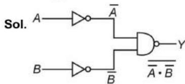
$$Y = \overline{\overline{A} \cdot \overline{B}} = A + B$$
